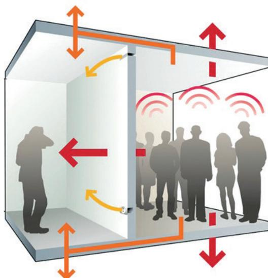
Noise transmission: -> direct / -> indirect or lateral / -> parasitic
